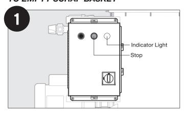
Ensure unit is turned off by pressing the STOP button on the control.
