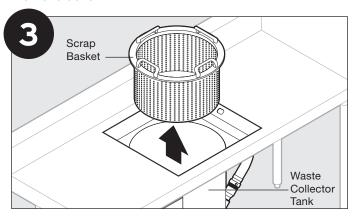
Remove scrap basket and dump waste into appropriate trash or compost receptacle.
