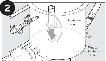
Place the overflow tube into the drain at the bottom of waste collector tank.
