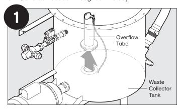
Turn off unit and empty scrap basket (see above instructions). Pull overflow tube to drain water inside waste collector tank.
