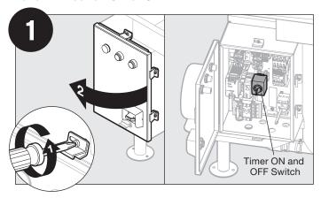
Open the control panel. Locate the Timer ON and OFF switch.
