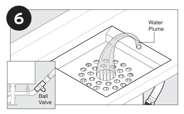
Adjust ball valve until water plume hits desired location inside tray area (recommended location is the center of scrap basket and/or cover).
