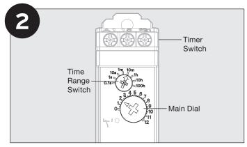
Rotate time range switch or main dial to desired settings (as shown). The time range switch sets the increments (0.1s, 1s, 10s, etc.) and the main dial is the "multiplier." The factory default is 10m on time range switch and 2 on the main dial, or 20 minutes.
