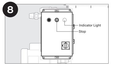
Press STOP on the control panel. Indicator light turns off.
