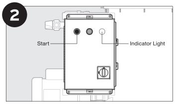
Press the START button. Indicator light turns on.
