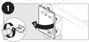
Remove top cover retainers by loosening screws and open the front panel.
