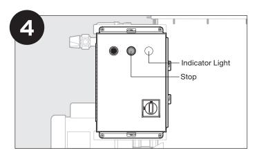
Turn off unit by pressing the STOP button. Indicator light turns off.
