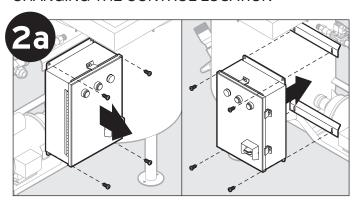
**Optional** – to relocate the control, remove and save four (4) bolts and nuts. Reposition box on other side of tank and secure with previously removed hardware. It is not necessary to disconnect factory-installed wiring.
