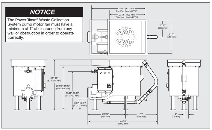
Figure 5. PowerRinse® Waste Collection System Dimensions
