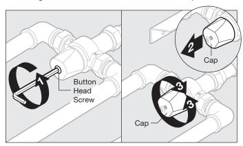
Figure 10. Adjusting Water Temperature
