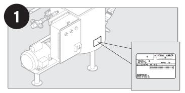
Remove unit from package. Ensure that the power supply is appropriate based on the control configuration ordered with the unit. Verify using spec plate on tank.
