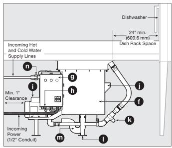
Figure 4. Typical Installation
