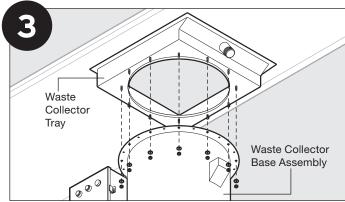
Secure waste collector base assembly to waste collector tray using provided lock washers and 1/4"-20 nuts.
