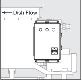
Verify dish flow and ensure that the control is on the proper side of the tank. The control should always face the operator and can be mounted on the opposite side of the tank if dish flow is reversed.
