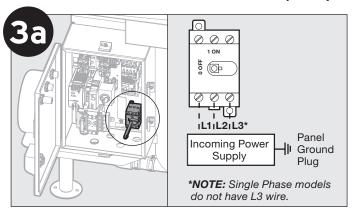
**For 3 Phase units only** – Ensure pump motor fan is rotating clockwise (when viewed from the motor end). If rotation is counter-clockwise, turn off power supply, open front panel, and switch L1 and L2 connections.
