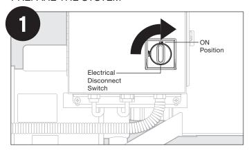
Turn electrical disconnect switch to the ON position. Open shutoff valves in water lines, if installed.
