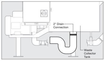
Figure 11. Drain Piping
