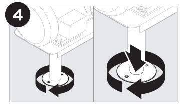
Rotate legs clockwise when viewing from top until they extend to the floor.
