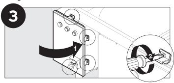
Close front panel and tighten screws on top cover retainers to secure.
