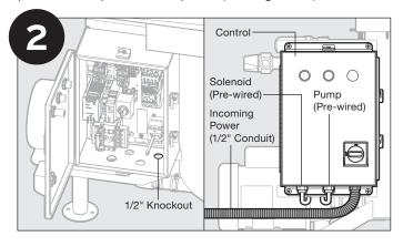
Run power from main power supply to the 1/2" knockout on bottom of control and connect as shown.
