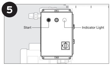
To begin, press START button on control and allow the reservoir tank to fill with water. Indicator light turns on. Pump turns on and water plume starts once tank has reached optimal fill level (approximately 70 seconds after pushing the START button).
