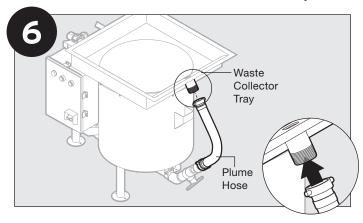
Connect plume hose to waste collector tray.
