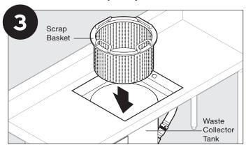
Place scrap basket inside waste collector tank. Unit must always have the scrap basket in place during operation.
