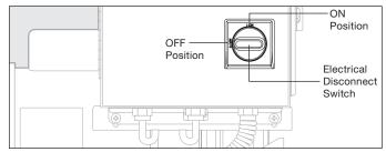
Figure 12. Electrical Disconnect Switch
