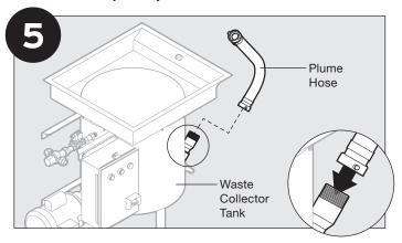
Connect plume hose to collector tank. Turn brass coupling clockwise to secure.
