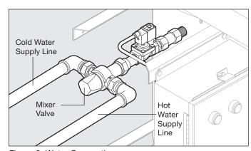
Figure 8. Water Connections
